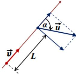
$$\Delta\varphi \equiv \omega \cdot \Delta t = \frac{u \cdot \sin(\alpha) \cdot \Delta t}{L} \Rightarrow \omega = \frac{u \cdot \sin(\alpha)}{L} = \frac{\sqrt{3}u}{2L} \approx 0,5000 \text{ с}^{-1}.$$
